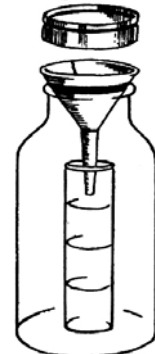
RUBBER BAND ROUND FUNNEL WHERE IT RESTS ON JAR. SO RAIN WON'T RUN DOWN OUTSIDE OF FUNNEL
